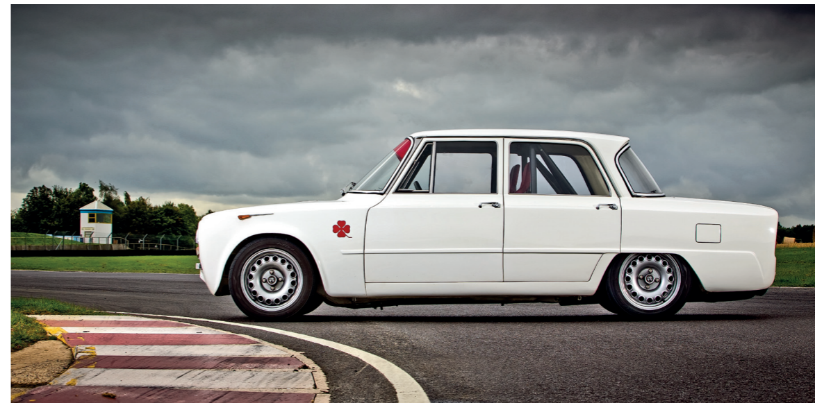
Above and left Ordinarily a Giulia saloon is about 100kg heavier than a GT Coupé – but this example has Perspex windows and carbonfibre bonnet and bootlid, which reduce the difference to only 25kg.
