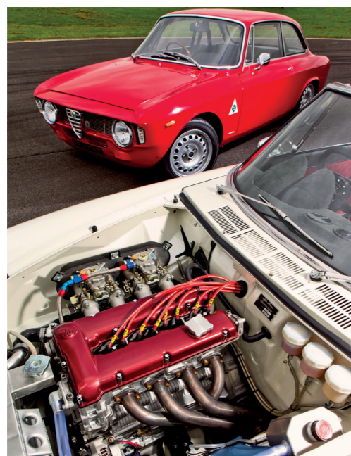
Right Twin Spark engine from a 1980s Alfa Romeo 75 looks period-correct in any of these 1960s models, thanks in part to Alfaholics' bespoke cam cover, but delivers a very non-period 216bhp.
