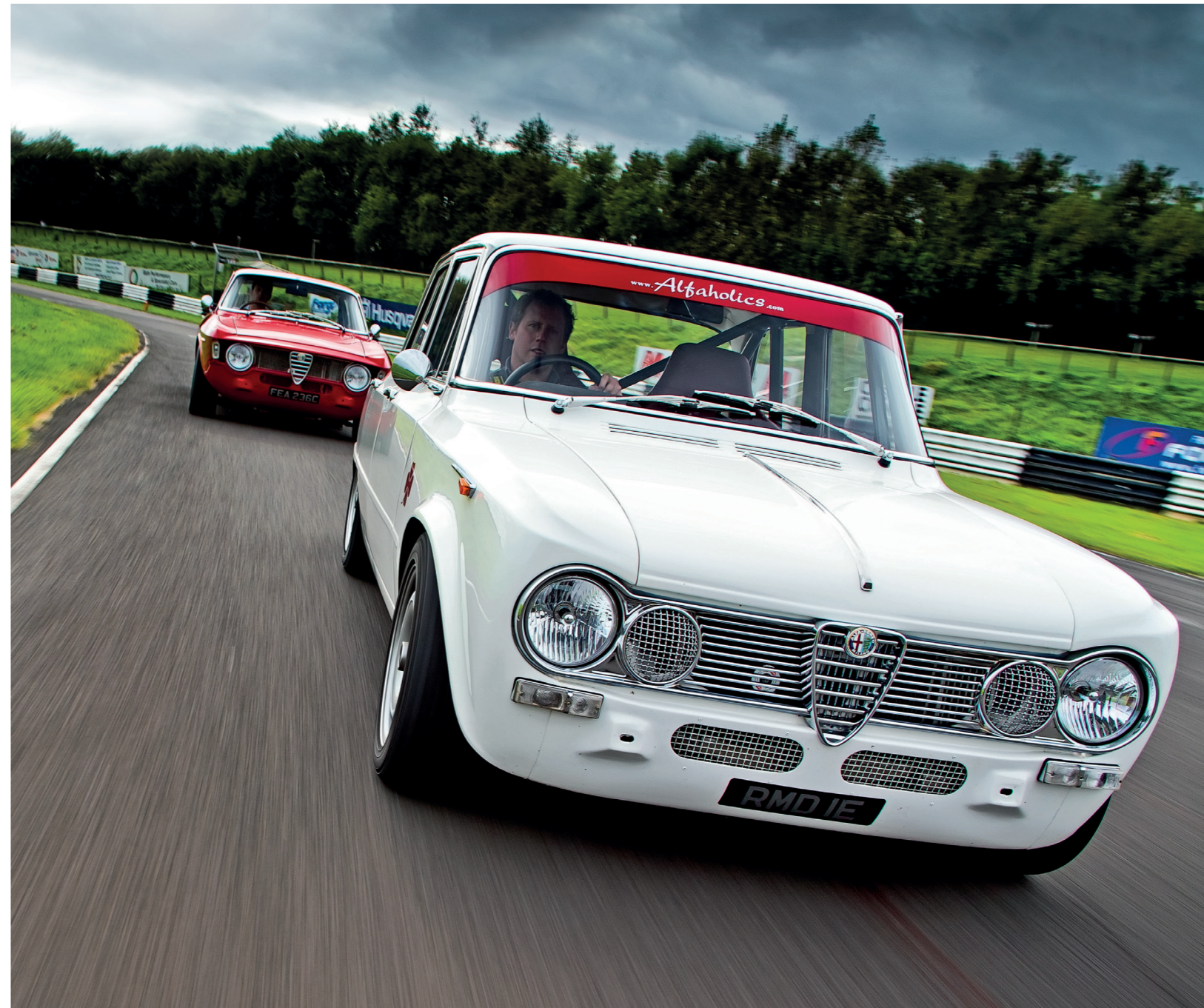
Above and left Ordinarily a Giulia saloon is about 100kg heavier than a GT Coupé – but this example has Perspex windows and carbonfibre bonnet and bootlid, which reduce the difference to only 25kg.
