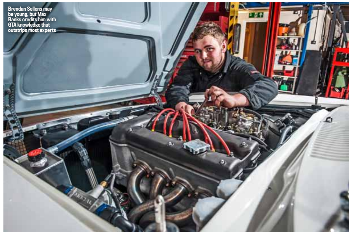
Twin-plug 1600 race engine is carb-fed; car had later 1300cc injection engine when found
