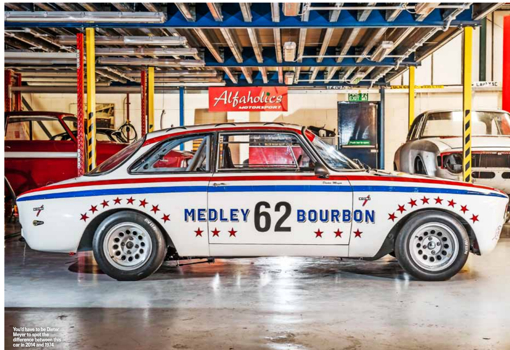
Front and rear wings were re-made before being cut back to fit bulging GRP arches
